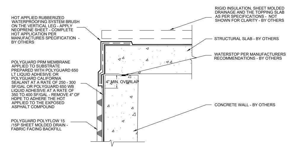
SECTION @ HOT APPLIED RUBBER TIE IN TO SELF ADHERED MEMBRANE
