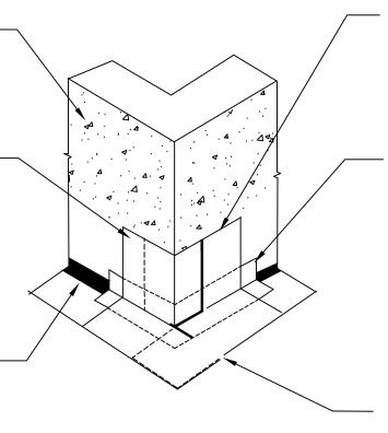
PIECE OF POLYGUARD PRM MEMBRANE CUT AND FIT TO OUTSIDE CORNER - APPLIED OVER SUBSTRATE PREPARED WITH POLYGUARD 650 LT LIQUID ADHESIVE OR POLYGUARD CALIFORNIA SEALANT AT A RATE OF 250 - 300 SF/GAL OR POLYGUARD 650 WB LIQUID ADHESIVE AT A RATE OF 350 - 400 SF/GAL
