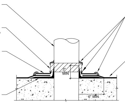
POLYGUARD DETAIL SEALANT PW OR POLYGUARD LM-95 APPLIED TO TERMINAL EDGES OF TARGET PATCH
