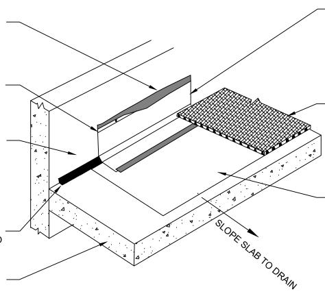
12" POLYGUARD DETAIL TAPE OR POLYGUARD 650 MEMBRANE APPLIED TO INSIDE AND **OUTSIDE CORNERS PREPARE** VERTICAL SUBSTRATE WITH POLYGUARD 650 LT LIQUID ADHESIVE OR POLYGUARD CALIFORNIA SEALANT AT A RATE OF 250 - 300 SF/GAL OR POLYGUARD 650 WB LIQUID ADHESIVE AT A RATE OF 350-400 SF/GAL AND ONTO EXISTING HORIZONTAL PRM MEMBRANE POLYGUARD POLYFLOW 18 SHEET MOLDED DRAIN OR PROTECTION -WOVEN MESH FACING TOPPING **SLAB**
