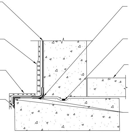
3/4" FILLET OF POLYGUARD DETAIL SEALANT PW OR POLYGUARD LM-95 APPLIED TO INSIDE CORNERS VERTICALLY AND HORIZONTALLY TO RAW CONCRETE - ALLOW POLYGUARD DETAIL SEALANT PW TO CURE FOR 2 HOURS PRIOR TO SHEET APPLICATION
