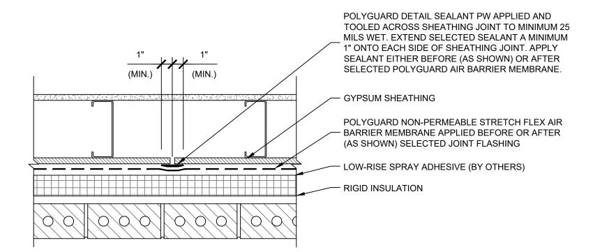
09 PLAN @ FRAMED BACKING WALL / MASONRY VENEER - SUBSTRATE JOINT
