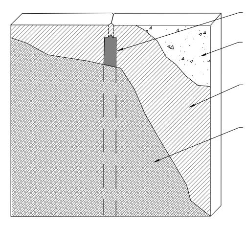
POLYGUARD DETAIL SEALANT PW APPLIED INTO CONTROL JOINT EXTENDING OUT ONTO THE FRONT FACE OF WALL A MINIMUM OF 1 1/2" AFTER POLYGUARD STRETCH FLEX IS CURED
