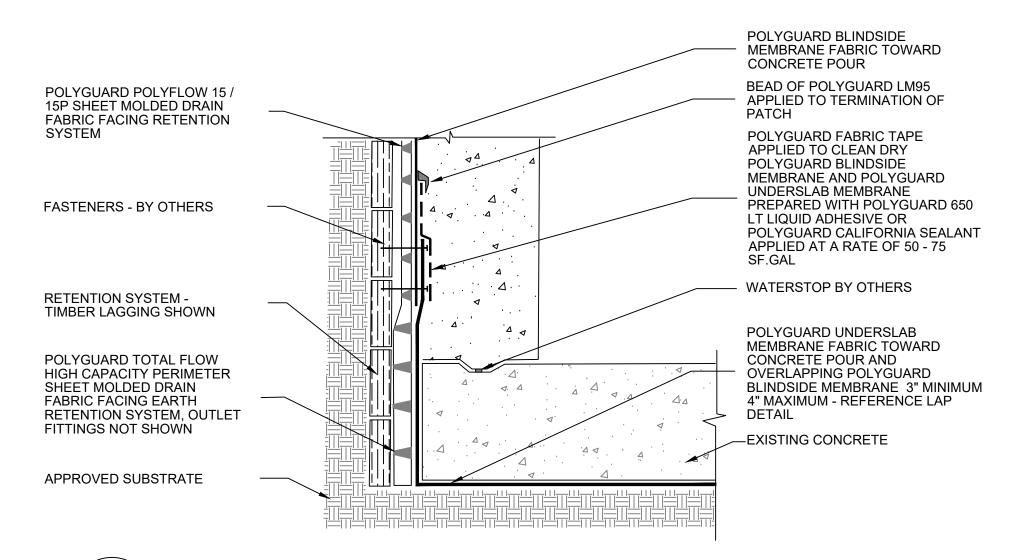
\_\_\_\_\_\_ US1 SECTION @ UNDERSLAB MEMBRANE TIE IN TO BLINDSIDE MEMBRANE
