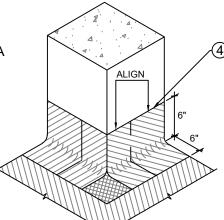
TOP EDGE OF POLYGUARD UNDERSLAB 'SKIRT' ALIGNED AND ADHERED TO TOP EDGE AND BODY OF POLYGUARD 606 TAPE AND THE EXPOSED BOOT COMPOUND. EXTEND FIELD LEG OF THE 'SKIRT' 6" ONTO THE FIELD MEMBRANE FABRIC AND EXPOSED BOOT COMPOUND.
