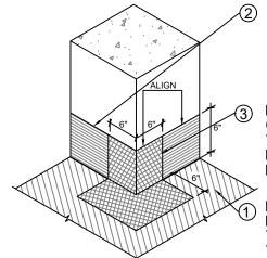
POLYGUARD 606 TAPE APPLIED TO CONCRETE PREPARED WITH POLYGUARD 650 LT LIQUID ADHESIVE OR POLYGUARD CALIFORNIA SEALANT APPLIED AT A RATE OF 250 - 300 SF / GAL
