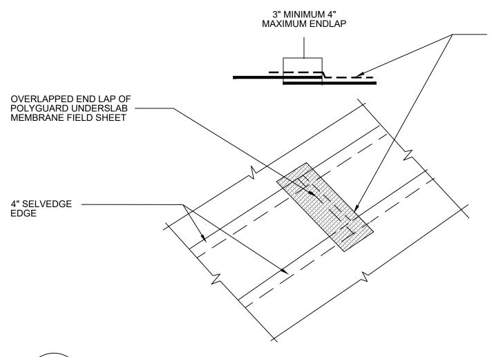
12" PIECE OF POLYGUARD FABRIC TAPE A MINIMUM 6" IN ALL DIRECTIONS PAST ENDLAP APPLIED TO CLEAN, DRY POLYGUARD UNDERSLAB MEMBRANE PREPARED WITH POLYGUARD 650 LT LIQUID ADHESIVE OR POLYGUARD CALIFORNIA SEALANT APPLIED AT A RATE OF 50 - 75 SF/GAL
