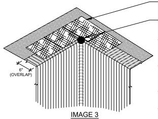
POLYGUARD FABRIC TAPE, EXTEND 6" TO EACH SIDE OF THE UNDERSLAB END LAP
