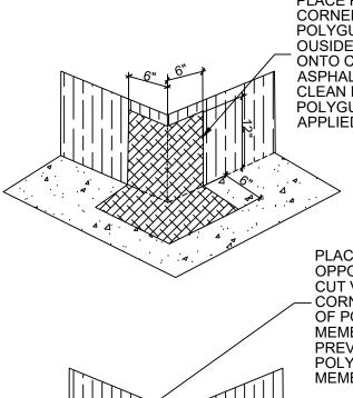
PLACE POLYGUARD OUTSIDE CORNER BOOT (REFERENCE POLYGUARD FIELD MADE OUSIDE CORNER BOOT DETAIL) ONTO CONCRETE FORM ASPHALT SIDE OUT - KEEP CLEAN FOR ADHESION OF POLYGUARD UNDERSLAB FIELD APPLIED CORNER PIECES
