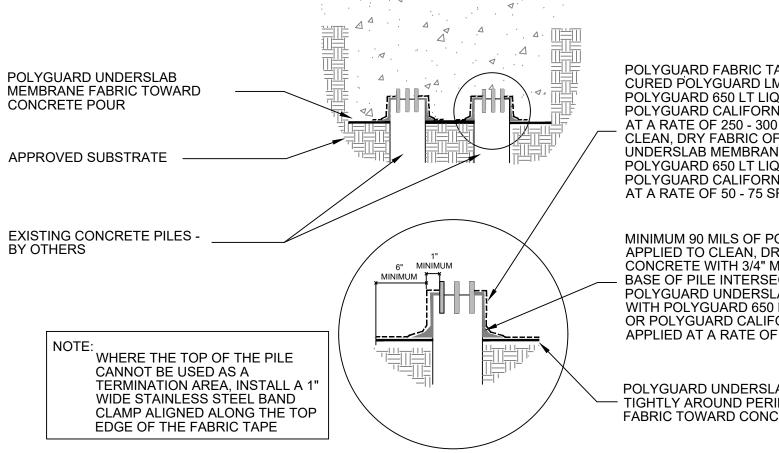
POLYGUARD FABRIC TAPE APPLIED OVER CURED POLYGUARD LM-95 PREPARED WITH POLYGUARD 650 LT LIQUID ADHESIVE OR POLYGUARD CALIFORNIA SEALANT APPLIED AT A RATE OF 250 - 300 SF/GAL AND ONTO CLEAN, DRY FABRIC OF POLYGUARD UNDERSLAB MEMBRANE PREPARED WITH POLYGUARD 650 LT LIQUID ADHESIVE OR POLYGUARD CALIFORNIA SEALANT APPLIED AT A RATE OF 50 - 75 SF/GAL
