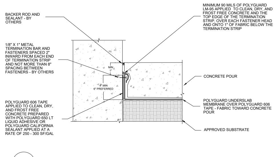
SECTION @ TERMINATION TO EXISTING CONCRETE WALL
