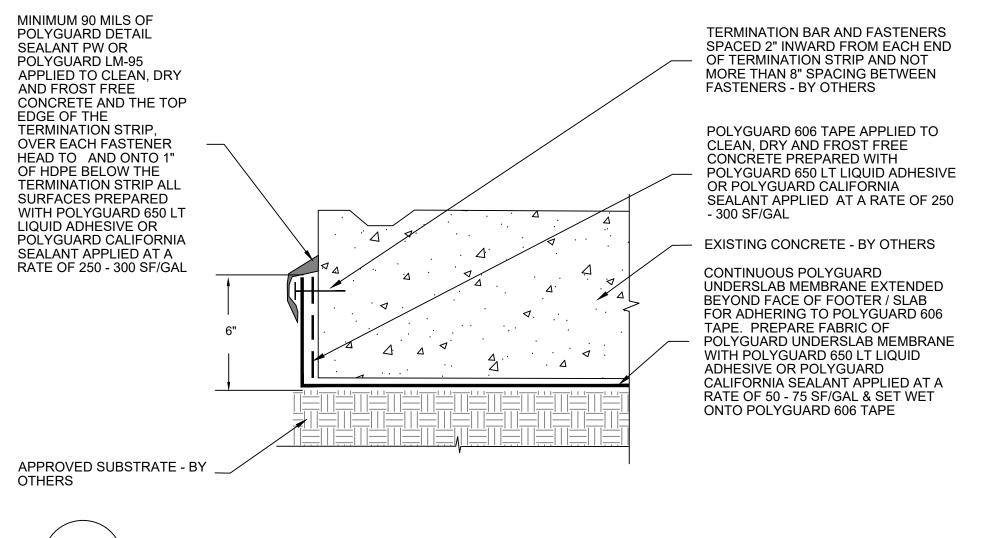
SECTION @ POST CONCRETE POUR TERMINATION TO FACE OF FOOTER - STRUCTURAL SLAB
