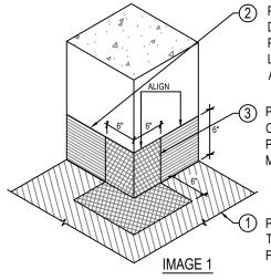
POLYGUARD 606 TAPE APPLIED TO CLEAN, DRY, FROST-FREE, RAW CONCRETE PREPARED WITH POLYGUARD 650 LT LIQUID ADHESIVE OR CALIFORNIA SEALANT APPLIED AT A RATE OF 250 - 300 SF / GAL
