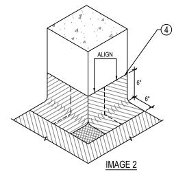
POLYGUARD UNDERSLAB TRM 'SKIRT' ALIGNED AND ADHERED TO TOP EDGE AND VERTICAL BODY OF POLYGUARD 606 TAPE AND PREFORMED US OUTSIDE CORNER BOOT EXPOSED COMPOUND; EXTEND MINIMUM 6" ONTO HORIZONTAL UNDERSLAB TRM FIELD SHEET FABRIC AND PREFORMED US OUTSIDE CORNER BOOT EXPOSED COMPOUND
