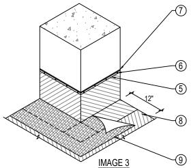
POLYGUARD LM-95 OR TRM SEALANT APPLIED TO MINIMUM 90 MILS OVER CLEAN. DRY, FROST-FREE, RAW CONCRETE; ALONG TERMINATION BAR TOP EDGE; OVER EACH FASTENER HEAD: AND EXTEND ONTO MINIMUM 1" OF POLYGUARD UNDERSLAB TRM FABRIC BELOW TERMINATION BAR PREPARED WITH POLYGUARD 650 LT LIQUID ADHESIVE OR CALIFORNIA SEALANT APPLIED AT A RATE OF 50 - 75 SF / GAL
