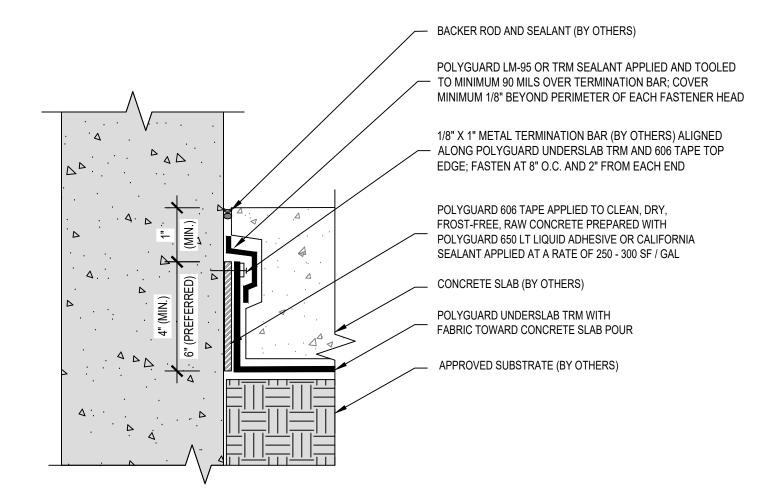
SECTION @ UNDERSLAB TRM - VERTICAL TERMINATION TO EXISTING CONCRETE FOUNDATION WALL
