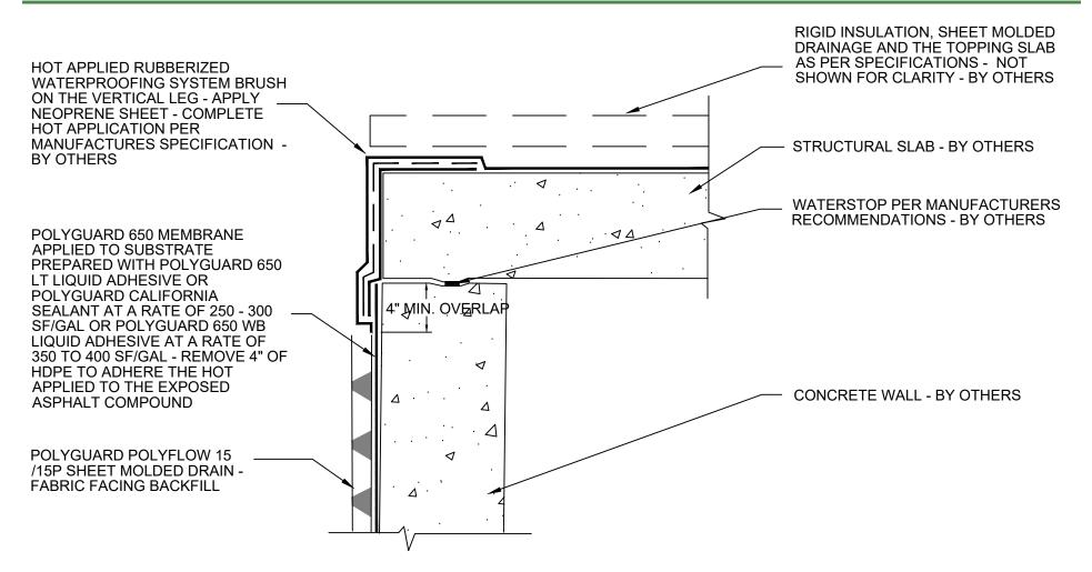
SECTION @ HOT APPLIED RUBBER TIE IN TO SELF ADHERED MEMBRANE WP12
