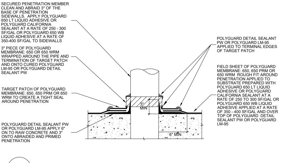
SECTION@ HORIZONTAL PENETRATION WATERPROOFING
