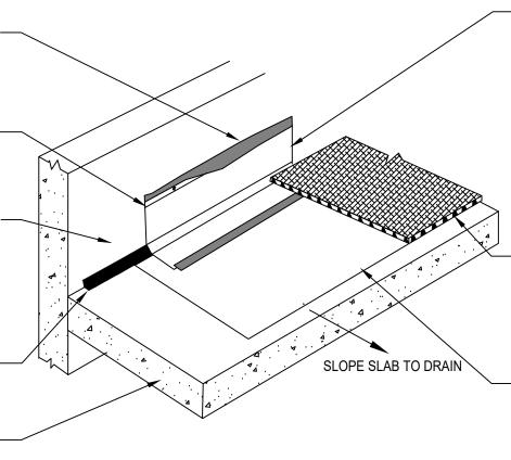
12" PIECE OF POLYGUARD DETAIL TAPE OR DETAIL TAPE WRM OR CUT PIECE OF POLYGUARD MEMBRANE: 650 OR 650 WRM APPLIED TO INSIDE AND OUTSIDE CORNERS PREPARE VERTICAL SUBSTRATE WITH POLYGUARD 650 LT LIQUID ADHESIVE OR POLYGUARD CALIFORNIA SEALANT AT A RATE OF 250 - 300 SF/GAL OR POLYGUARD 650 WB LIQUID ADHESIVE AT A RATE OF 350-400 SF/GAL AND ONTO EXISTING HORIZONTAL POLYGUARD MEMBRANE: 650, 650 PRM OR 650 WRM
