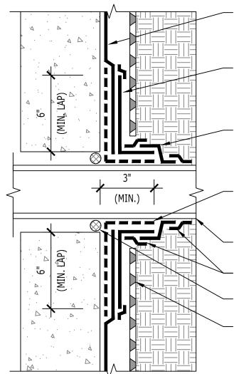
POLYGUARD 650 TRM; ROUGH-FIT AROUND PENETRATION AND OVER POLYGUARD TRM SEALANT PREPARED WITH POLYGUARD 650 LT LIQUID ADHESIVE OR CALIFORNIA SEALANT APPLIED AT A RATE OF 250 - 300 SF / GAL, OR OVER 650 WB LIQUID ADHESIVE APPLIED AT A RATE OF 350 - 400 SF / GAL
