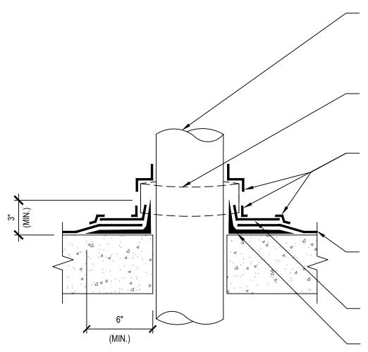
SECURED PENETRATION MEMBER, CLEAN AND ABRADE MINIMUM 3" OF BASE OF PENETRATION SIDEWALLS. APPLY POLYGUARD 650 LT LIQUID ADHESIVE OR CALIFORNIA SEALANT AT A RATE OF 250 - 300 SF / GAL, OR POLYGUARD 650 WB LIQUID ADHESIVE APPLIED AT A RATE OF 350-400 SF / GAL, TO SIDEWALLS TO PRIME FOR SHEET MEMBRANE OVERLAY APPLICATION
