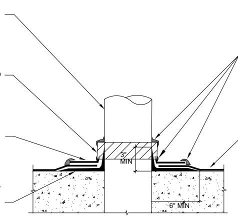
POLYGUARD DETAIL SEALANT PW OR POLYGUARD LM-95 APPLIED TO TERMINAL EDGES OF TARGET PATCH
