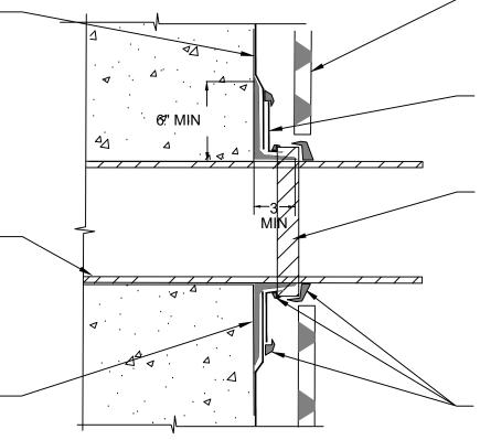
POLYGUARD POLYFLOW 15 / 15P SHEET MOLDED DRAIN
