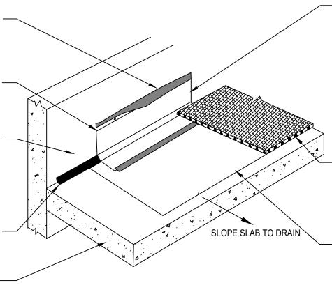
12" PIECE OF POLYGUARD DETAIL TAPE OR DETAIL TAPE WRM OR CUT PIECE OF POLYGUARD MEMBRANE: 650 OR 650 WRM APPLIED TO INSIDE AND OUTSIDE CORNERS PREPARE VERTICAL SUBSTRATE WITH POLYGUARD 650 LT LIQUID ADHESIVE OR POLYGUARD CALIFORNIA SEALANT AT A RATE OF 250 - 300 SF/GAL OR POLYGUARD 650 WB LIQUID ADHESIVE AT A RATE OF 350-400 SF/GAL AND ONTO EXISTING HORIZONTAL POLYGUARD MEMBRANE: 650, 650 PRM OR 650 WRM
