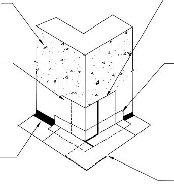
PIECE OF POLYGUARD MEMBRANE: 650 OR 650 WRM CUT AND FIT TO OUTSIDE CORNER - APPLIED OVER SUBSTRATE PREPARED WITH POLYGUARD 650 LT LIQUID ADHESIVE OR POLYGUARD CALIFORNIA SEALANT AT A RATE OF 250 - 300 SF/GAL OR POLYGUARD 650 WB LIQUID ADHESIVE AT A RATE OF 350 - 400 SF/GAL
