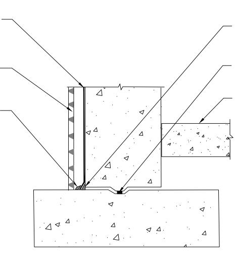
3/4" FACE OF POLYGUARD DETAIL SEALANT PW OR POLYGUARD LM-95 FILLET /CANT
