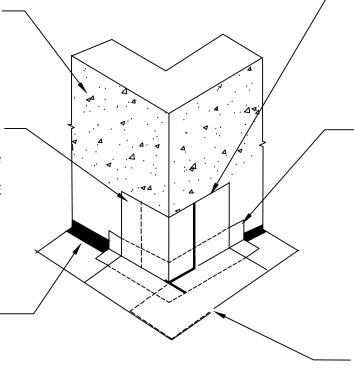
PIECE OF POLYGUARD 650 MEMBRANE CUT AND FIT TO OUTSIDE CORNER - APPLIED OVER SUBSTRATE PREPARED WITH POLYGUARD 650 LT LIQUID ADHESIVE OR POLYGUARD CALIFORNIA SEALANT AT A RATE OF 250 - 300 SF/GAL OR POLYGUARD 650 WB LIQUID ADHESIVE AT A RATE OF 350 - 400 SF/GAL
