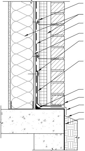
WALL TIE, FASTENER HOLE SEALED AND TOOLED WITH POLYGUARD DETAIL SEALANT PW BETWEEN BACK OF WALL TIE AND AIR BARRIER FIELD MEMBRANE
