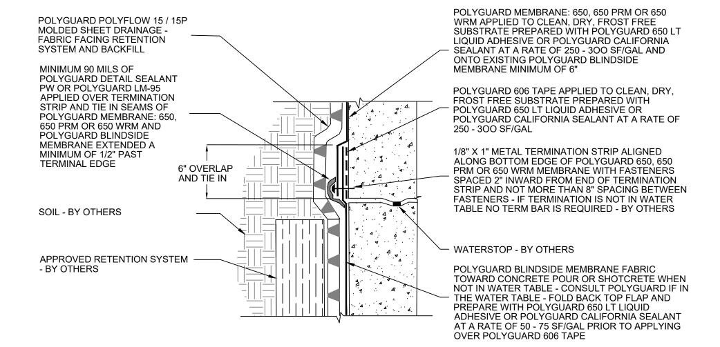
SECTION @ VERTICAL TERMINATION OF 650 / 650 PRM / 650 WRM TO BLINDSIDE MEMBRANE
