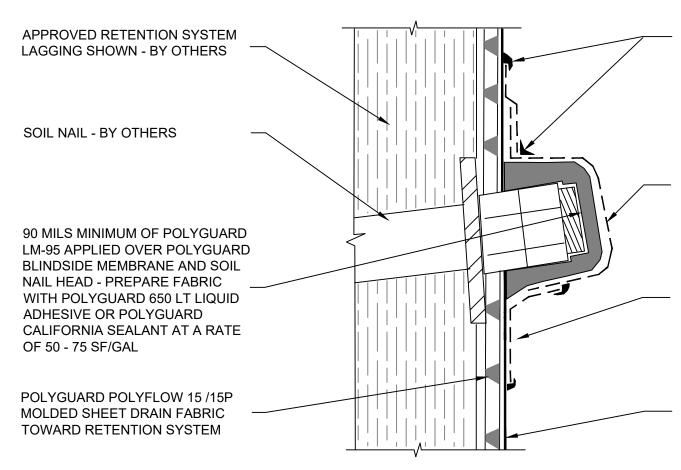
POLYGUARD DETAIL SEALANT PW OR POLYGUARD LM-95 APPLIED OVER TERMINATION OF POLYGUARD FABRIC TAPE AND ONTO POLYGUARD BLINDSIDE MEMBRANE - PREPARE FABRIC WITH POLYGUARD 650 LT LIQUID ADHESIVE OR POLYGUARD CALIFORNIA SEALANT AT A RATE OF 50 - 75 SF/GAL
