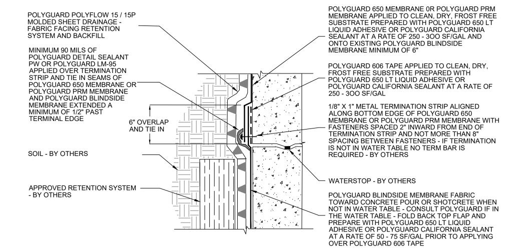
SECTION @ VERTICAL TERMINATION OF 650 / PRM TO BLINDSIDE MEMBRANE
