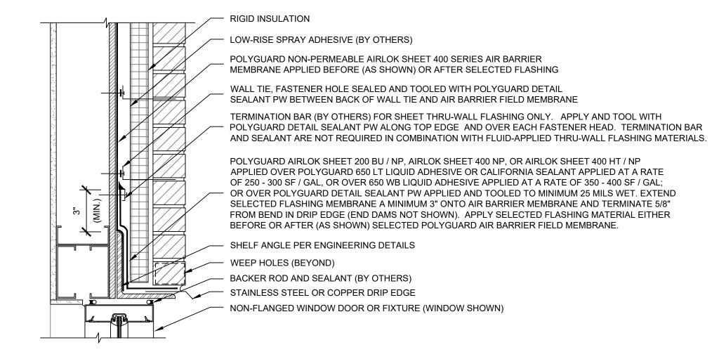
SECTION @ FRAMED BACKING WALL / MASONRY VENEER - NON-FLANGED WINDOW, DOOR, OR FIXTURE HEAD
