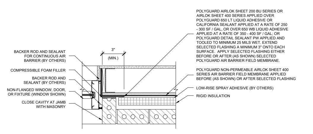
04 PLAN @ FRAMED BACKING WALL / MASONRY VENEER - NON-FLANGED WINDOW, DOOR, OR FIXTURE JAMB ©POLYGUARD PRODUCTS, INC
