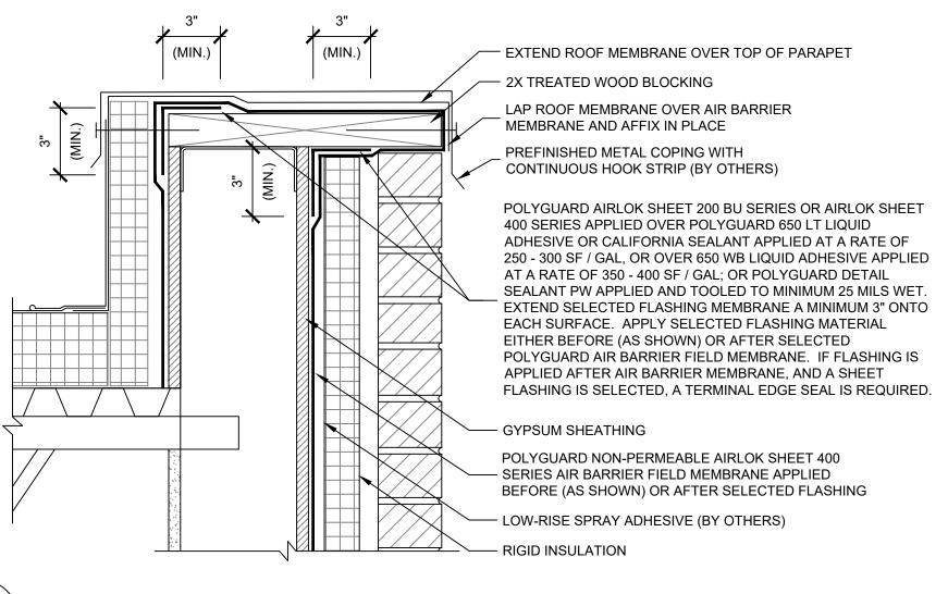
SECTION @ FRAMED BACKING WALL / MASONRY VENEER - PARAPET
