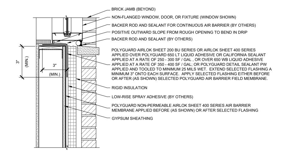
05 SECTION @ FRAMED BACKING WALL / MASONRY VENEER - NON-FLANGED WINDOW, DOOR, OR FIXTURE SILL
