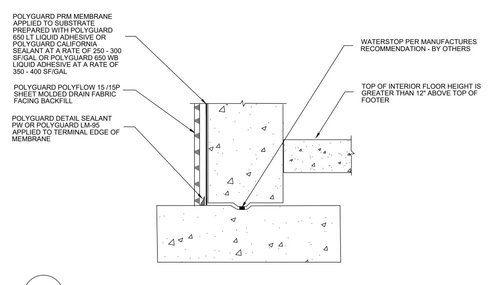
PRM10 SECTION @ TOP OF INTERIOR FLOOR GREATER THAN 12" FROM TOP OF FOOTER
