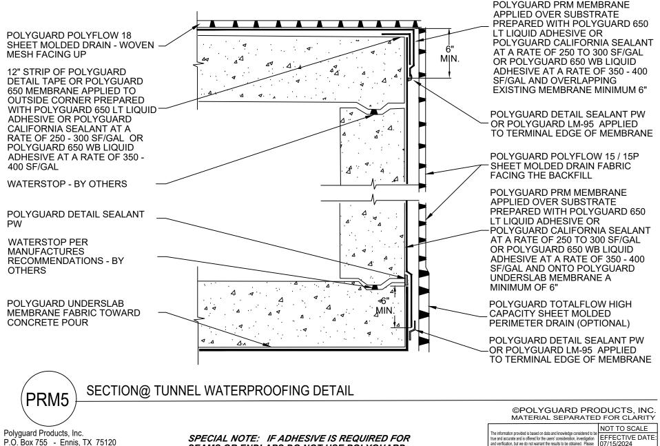
P.O. Box 755 - Ennis, TX 75120 Phone: 214-515-5000 Web Site - www.polyguard.com SPECIAL NOTE: IF ADHESIVE IS REQUIRED FOR SEAMS OR ENDLAPS DO NOT USE POLYGUARD 650 WB LIQUID ADHESIVE
