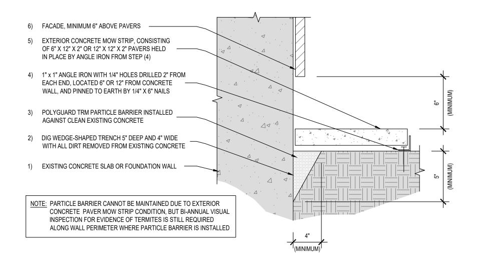
SECTION @ TRM PARTICLE BARRIER - UNDER MOW STRIP ADJACENT TO EXISTING CONCRETE STRUCTURE
