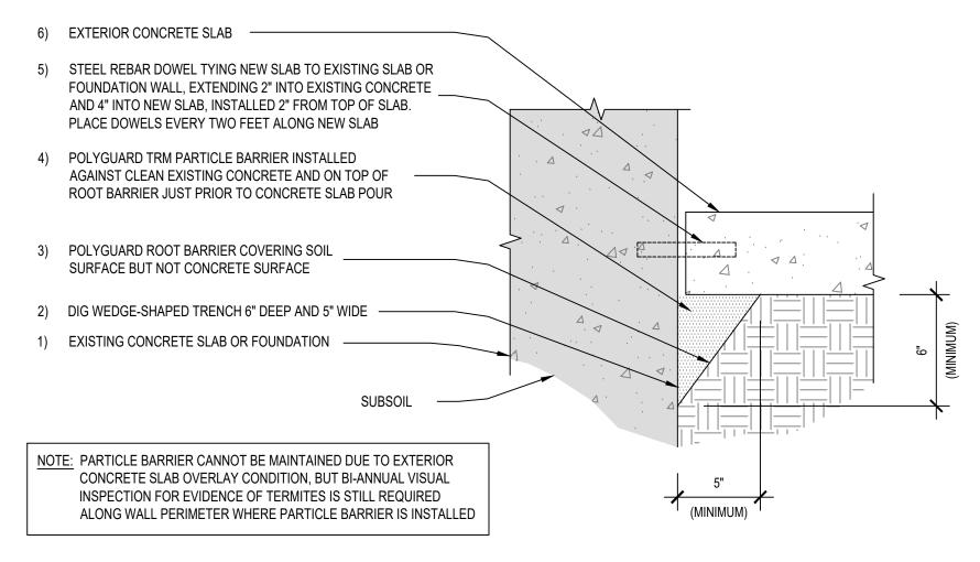
SECTION @ TRM PARTICLE BARRIER UNDER CONCRETE SLAB (DRIVEWAY, PATIO OR SLAB) ADJACENT TO EXISTING CONCRETE STRUCTURE
