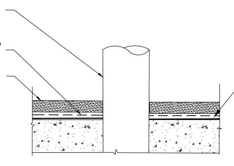
40 MILS OF POLYGUARD LM85 SSL APPLIED TO CLEAN DRY SUBSTRATE MUST APPLY UP TO AND TOUCHING THE PIPE
