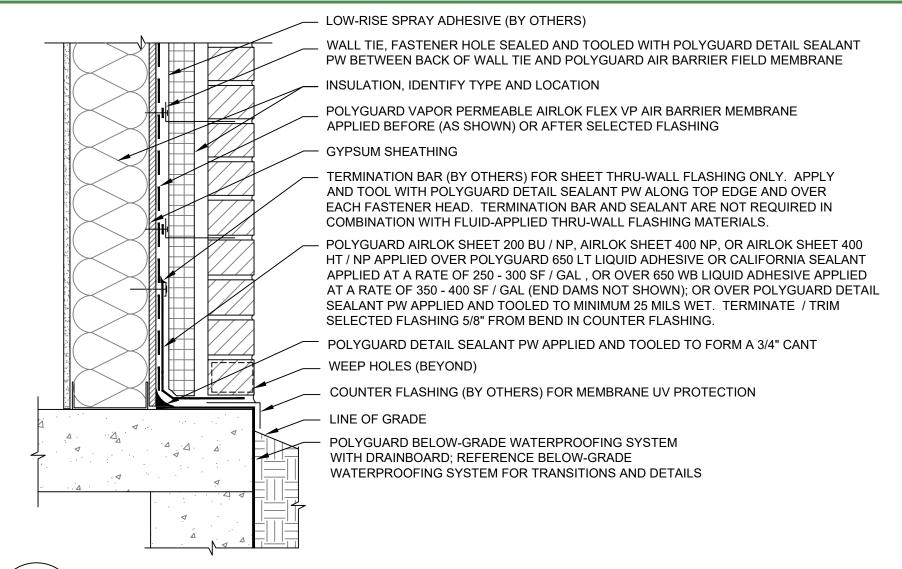
01 \SECTION @ FRAMED BACKING WALL / MASONRY VENEER - WALL BASE
