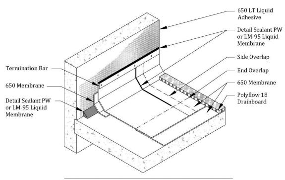
650 Membrane Horizontal Slab Wall Termination
