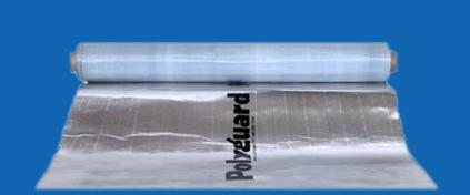
Ultra CRM™ - Chemical Resistant Membrane - is a strong, 60-mil, post-applied membrane designed and tested to withstand elevated concentrations of soil, fluid and vapor contaminants when installed on below grade concrete or CMU structures; such as concrete foundation walls, tunnels, parking garages and related applications where chemical resistant waterproofing is critical.
