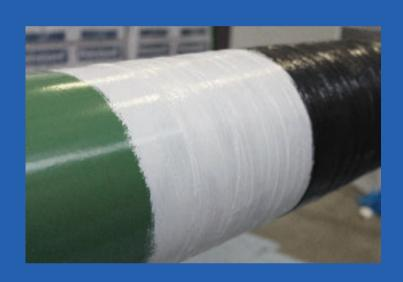
RD-6 UVO is an Ultra Violet Overcoat which is highly resistant to the damaging effects of UV light. It is a single component, low VOC, water based liquid coating that protects RD-6 anti-corrosion coating from harmful UV rays. Direct exposure to sunlight will result in degradation of the RD-6. RD-6 UVO should be used as an overcoat to protect RD-6 on above ground pipeline field joint girth welds, valves, fittings, and FBE coated pipe from damaging UV light rays.
