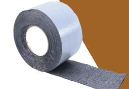
Polyguard RD-6® Coating System is a non-shielding anti-corrosion system used on buried and submerged line pipe, rehabilitation and new construction girth welds. RD-6 can also be used above ground but the coating must be protected from harmful UV rays by using RD-6 UV Overcoat. It consists of a liquid adhesive, a geotextile backed protective pipeline coating and SP-6 outerwrap. RD-6 is compatable for pipelines operating up to 145°F (63°C); for pipes operating above 145°F, RD-6 HT must be used.
