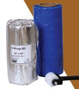
X-Wrap HD (formerly IRO HD - Impact Resistant Outerwrap-Heavy Duty) is designed to protect field joint coatings and mainline coatings from abrasion and mechanical damage. X-Wrap HD consists of pre-impregnated woven glass fabric and water activated resin. This product is designed for use during tunneling, horizontal directional drilling (HDD) and bores. X-Wrap HD supersedes IRO HD products and should be substituted for all future use.
