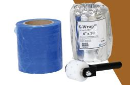
X-Wrap (formerly IRO - Impact Resistant Outerwrap) is designed to protect field joint coatings and mainline coatings from abrasion and mechanical damage. X-Wrap consists of pre-impregnated woven glass fabric and water activated resin. This product is designed for use during tunneling, horizontal directional drilling (HDD) and bores. X-Wrap supersedes IRO and should be substituted for all future use.
