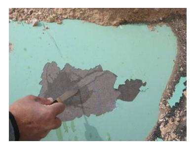
This disbonded FBE had no corrosion underneath. The pH of the water under the blister was elevated (made more alkaline) as the result of the CP currents being able to reach underneath the disbondment.
