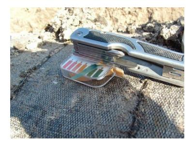
Water underneath a disbonded area of this improperly applied RD-6® had a pH of 9-10, as compared to water under nearby disbonded coal tar coating, which has a pH of 5-6. The CP current had increased the alkalinity of the water under the RD-6® to a level which does not support corrosion.
