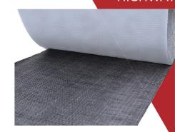
Polyguard 665 Membrane is a part of Polyguard's Highway family of products, and is a 65 mil membrane composed of a self-adhering, rubberized asphalt layer, laminated to a woven polypropylene backing. 665 Membrane is easy to work with and equally effective on bridges and pavements for waterproofing and crack control.
