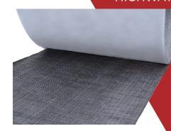
Polyguard 665 Membrane is a part of Polyguard's Highway family of products, and is a 65 mil membrane composed of a self-adhering, rubberized asphalt layer, laminated to a woven polypropylene backing. 665 Membrane is easy to work with and equally effective on bridges and pavements for waterproofing and crack control.
