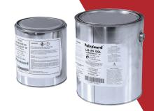
Polyguard LM 85 SSL is a part of Polyguard's Highway family of products, and is a two component, semi-self-leveling, asphalt modified urethane liquid membrane for use on new and repaired concrete. 45 minute working time. Useful for leveling out uneven substrate conditions on bridge deck applications.
