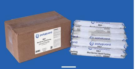
Blue Barrier™ Liquid Flashing is an all-purpose, fluid-applied flashing installed with an application gun and trowel used to create a weather resistant, fully adhered air barrier system around window and door installations. It was developed utilizing Silyl Terminated Polyether Technology (STPE). It comes in a 20oz "sausage tube" requiring a "sausage gun" to apply. Can be left exposed to UV light for up to 9 months.
