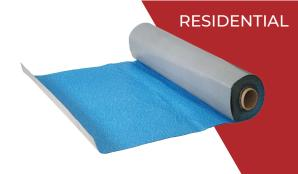
Deckguard® HT is a high heat 40-mil roofing membrane composed of a high strength slip resistant spider web backing laminated to a high performance high heat asphalt compound with a film release for ease of application. The release liner is removed leaving a strong asphalt compound to bond to the roof deck.
