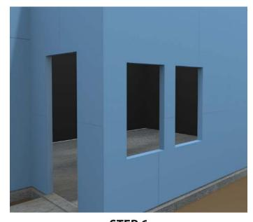
**STEP 6**Completely cover the entire wall substrate (OSB) around the entire above grade portion of the building.
