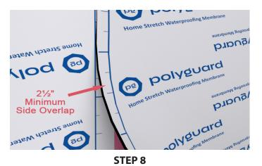
Home Stretch 40 Mil Membrane side laps shall be 2-1/2 inches minimum. Staggered end laps shall be 6 inches minimum.
