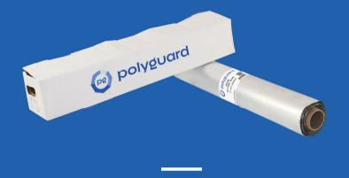
UV 2-Year 40 Mil is arubberized asphalt waterproofing sheet membrane, laminated to two layers of high strength polyethylene film, with a top protective layer of aluminum.
