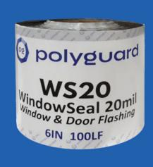
WindowSeal 20 Mil Flashing Tapes are used to strip in or flash straight window frames, door frames, and other construction seams. WS20 is a self-adhering, self-sealing tape consisting of rubberized asphalt waterproofing coating, laminated to polyethylene film. The finished product is supplied in rolls, with an easy to remove film release liner. WS20 is available in 20 mil thickness and a variety of roll sizes.
