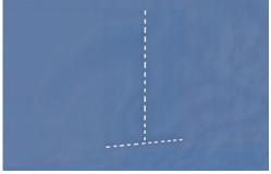
STEP 2B - Option B Cut the WRB at the bottom of the rough opening horizontally with your utility knife from side to side and then again down the middle of the window opening.
