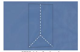
STEP 2A - Option A Cut an inverted "Y" in the WRB folding and secure it to the inside at the jambs and sill. In the middle of your rough opening, cut the WRB down to the left corner of the opening. Repeat on the right side, creating a "triangular" cut. Go to the top center of the opening and cut straight down to the top of
