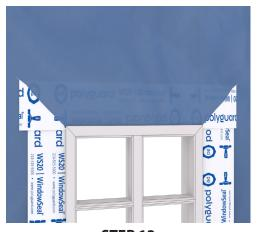
STEP 13 Fold the WRB back in place over the WS20 head flashing and secure with WS20.
