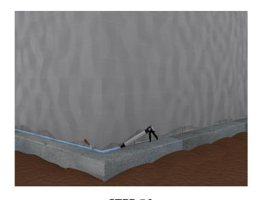
**STEP 5A**Apply a 3/4-inch, tooled bead of Blue Barrier Gap Filler at the intersection of the vertical foundation wall and the horizontal footer face prior to the Stretch Flex application.
